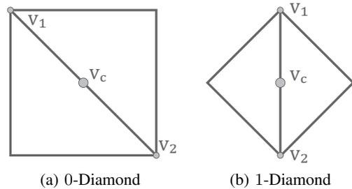
**Figure 1: The two classes of diamonds. In both cases, the spine is the internal edge with extreme vertices  $\mathbf{v}_1$  and  $\mathbf{v}_2$  and the central vertex  $\mathbf{v}_c$  is located at the midpoint of the spine.**
