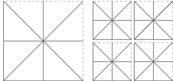
**Figure 3: Super-squares are sets of edges that tile each level of resolution within the hierarchy. The super-squares on the right are one level of resolution higher than the one on the left.**
