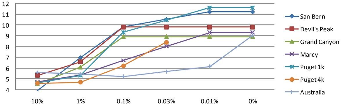
**Figure 5: Average density of super-squares (vertical axis) with uniform error (horizontal axis). Derived from Table 2 as  $(|\delta|/|\sigma|)$ .**
