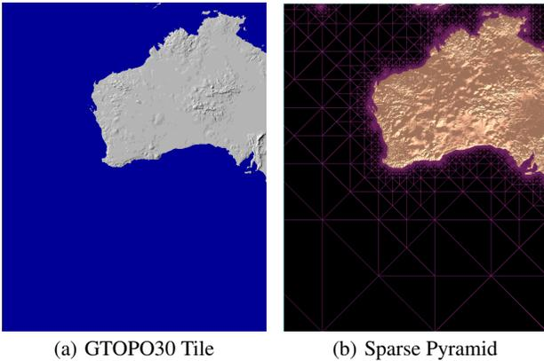
**Figure 2: Terrains covering large flat regions such as oceans are oversampled by a regular grid (a). A zero error sparse representation of this terrain (b) requires less than 1/6 of the samples from the original dataset. Image (a) courtesy of USGS [22].**
