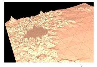
Figure 20: An RSB mesh extracted from the 1025<sup>2</sup> sample Puget Sound dataset using a circular *region of interest* query.
