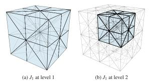
Figure 16: Each level of resolution within an RSB hierarchy is tiled by scaled fully-subdivided cubes. Two consecutive levels of resolution covering the same 3D domain are shown, containing 1 and 8 fully-subdivided cubes.
